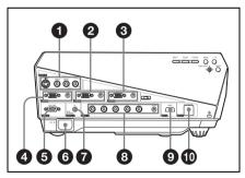
VIDEO IN (Video input) Connects to external video equipment . S VIDEO (mini DIN 4-pin) Connects to the S video output (Y/C video output) of video equipment. VIDEO (phono type)
