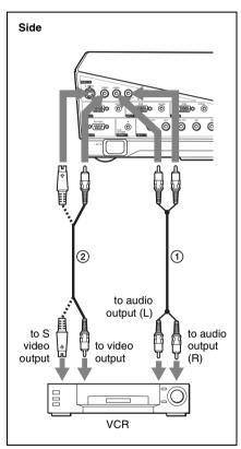
① Audio connecting cable (not supplied) For stereo equipment use both the L and R jacks.
