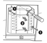
5 Insert the new lamp all the way in until it is securely in place (1). Tighten the two screws (2).
